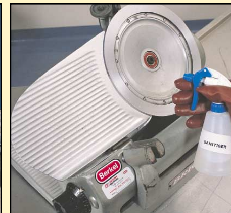
Spray machine with solution of sanitiser and leave to soak as per manufacturer's instructions. Rinse machine in clean water.
