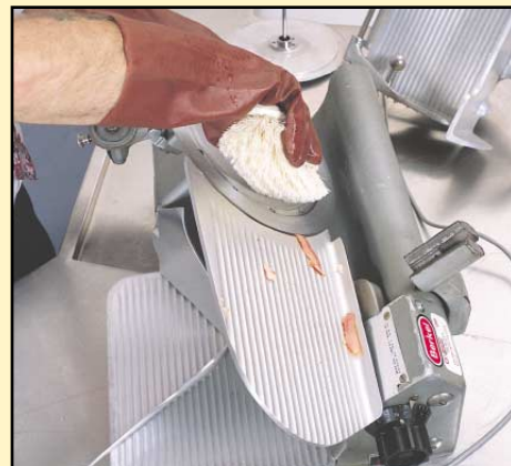
Use a dry brush to remove loose crumbs from machine and parts.
