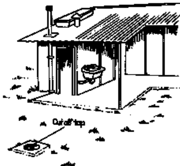
Fig. 6.25: House cut-off tap.
