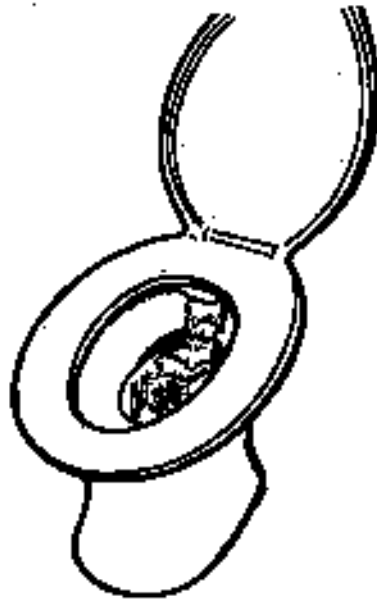
Fig. 2.10:Water continually flowing into the pedestal pan means there is something wrong with the cistern.
