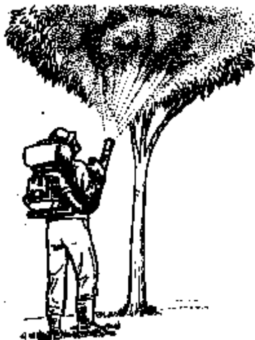
Fig. 5.29: Motorised back pack sprayer.
